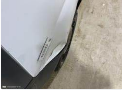
5 - Wing trim RR - Missing
