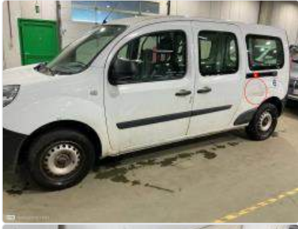
3 - Wing RL - Dent(s) and scratch(es)
