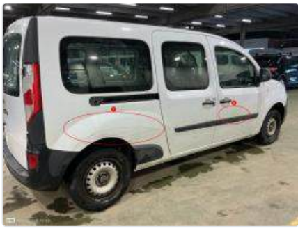
3 - Wing RL - Dent(s) and scratch(es)
